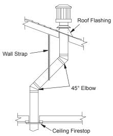
Figure 15 - Offset with Wall Strap and 45° Elbows
